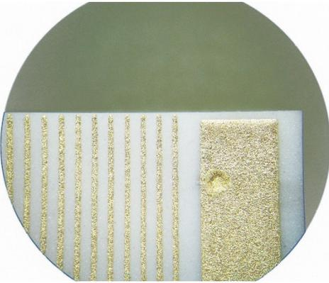
Gold Etched Thick Film with Plugged Via
