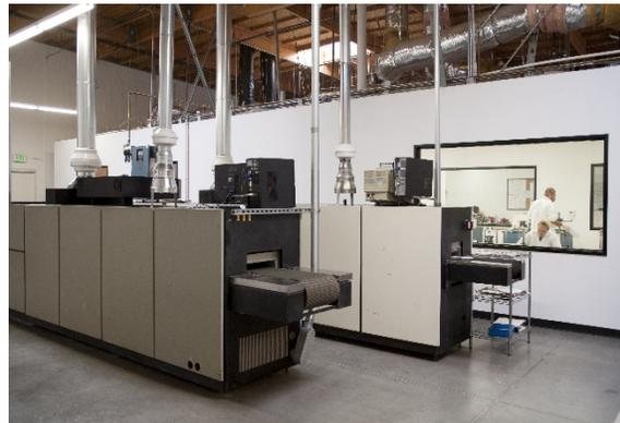
Belt Furnaces for Thick Film Firing
