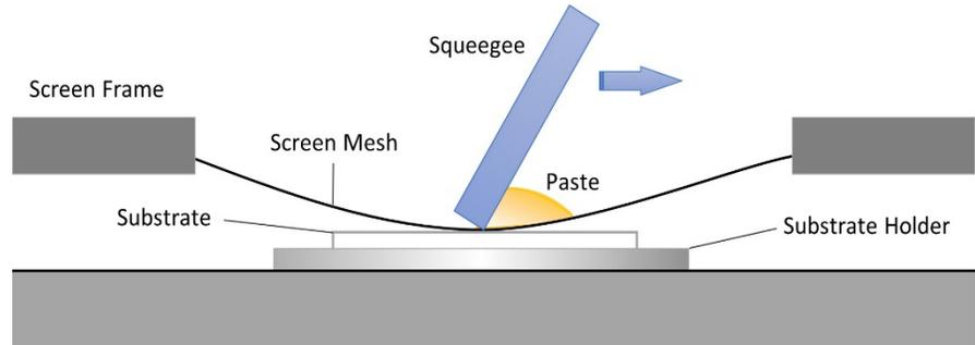
Additive Thick Film Screen Printing Process
