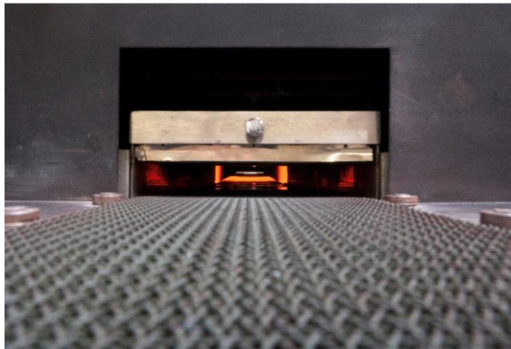
Firing at 850°C allows for all volatile contaminants to be fired and removed from the circuit
